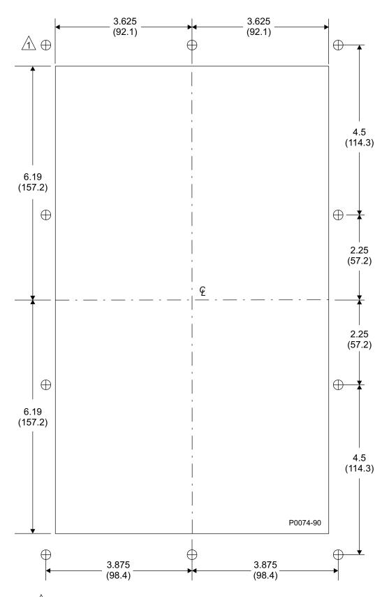
Mounting holes (10 places) are 0.218 (5.54) diameter. Use provided hardware when attaching escutcheon plate to DECS-250N.
